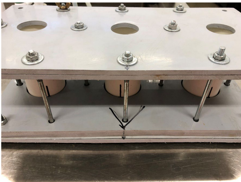
Figure 3 Test apparatus and weighing of Aquaproof 115 UV-R - Waterproofing Membrane
